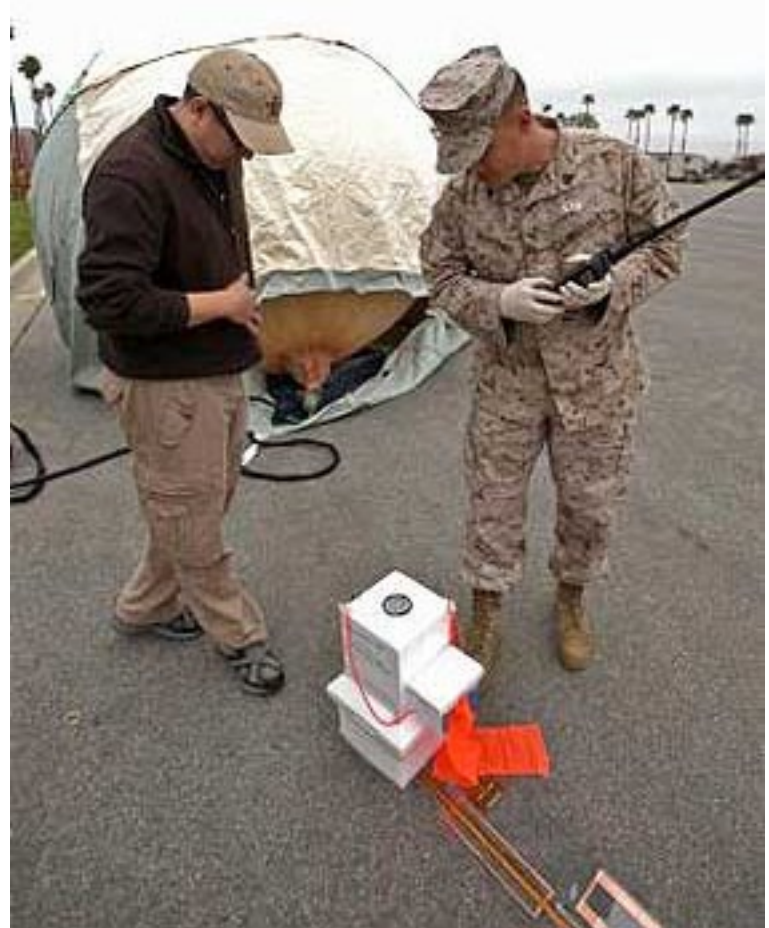
Pyisone Win, project manager, Space Data Corporation, and Sgt. Emmanuel T. Martinez, radio supervisor, Command Element, 15th Marine Expeditionary Unit, prepare the Combat SkySat communication system at Camp Pendleton, California, March 29, before allowing the helium balloon to float to Earth's stratosphere. The SkySat system is used to retransmit UHF signals to increase the range of communication up to 600 miles in diameter and expands the capabilities of the Marine Air Ground Task Force.
