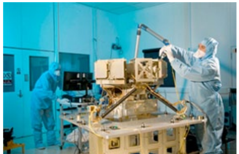
MIRI during ambient temperature alignment testing at the Science and Technology Facilities Council's Rutherford Appleton Laboratory, in the U.K. Image credits: STFC / Stephen Kill
