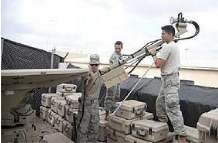
Tactical Networking technicians from the Combined Joint Task Force - Horn of Africa's communications directorate assemble an access point satellite terminal here April 19. These terminals, operated by the TACNET section, provides U.S. troops a secure medium for communications in support of CJTF-HOA missions. Photo by Staff Sgt. Andrew Caya
