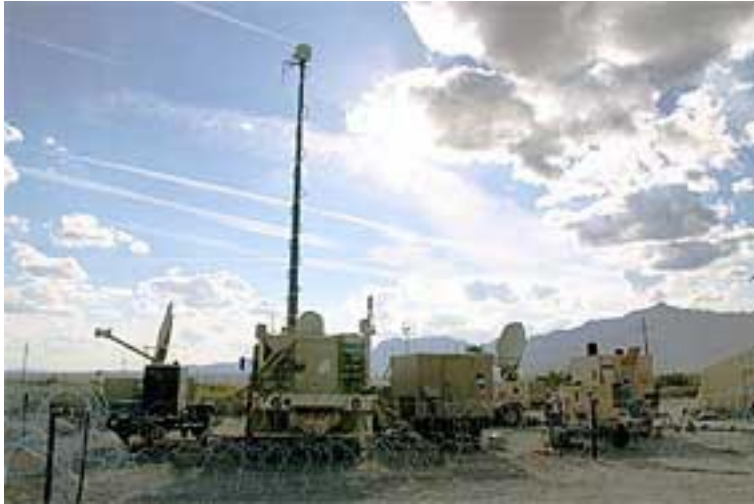
Warfighter Information Network-Tactical (WIN-T) equipment is pictured in preparation for the Army's Network Integration Evaluation 12.1 in November 2011. Second from left is a WIN-T Increment 2 Tactical Communications Node (TCN). (Photo courtesy: Claire Schwerin, U.S. Army)
