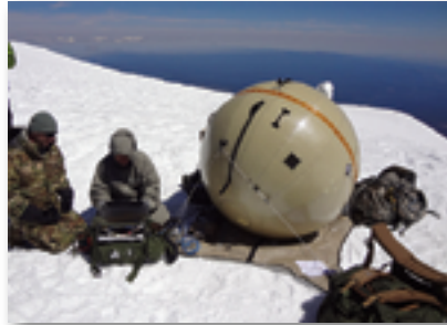
Ground to Air Transmit and Receive Inflatable Satellite Antennas are increasing agility and expeditionary nature of U.S. forces. U.S. Army photo.
