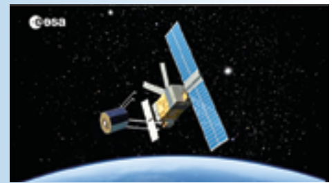
Simulations of orbital debris show that actively removing large items of debris, such as entire derelict satellites, should help stabilize its population and prevent a collision-based cascade effect. ESA has performed a system study for an Active Debris Removal mission called e.Deorbit. Image courtesy of ESA.
