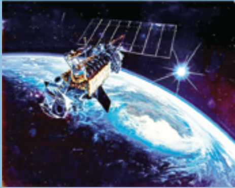
A U.S. Air Force Defense Meteorological Satellite Program (DMSP) satellite, a military weather satellite located in LEO. Image courtesy of U.S.A.F.
