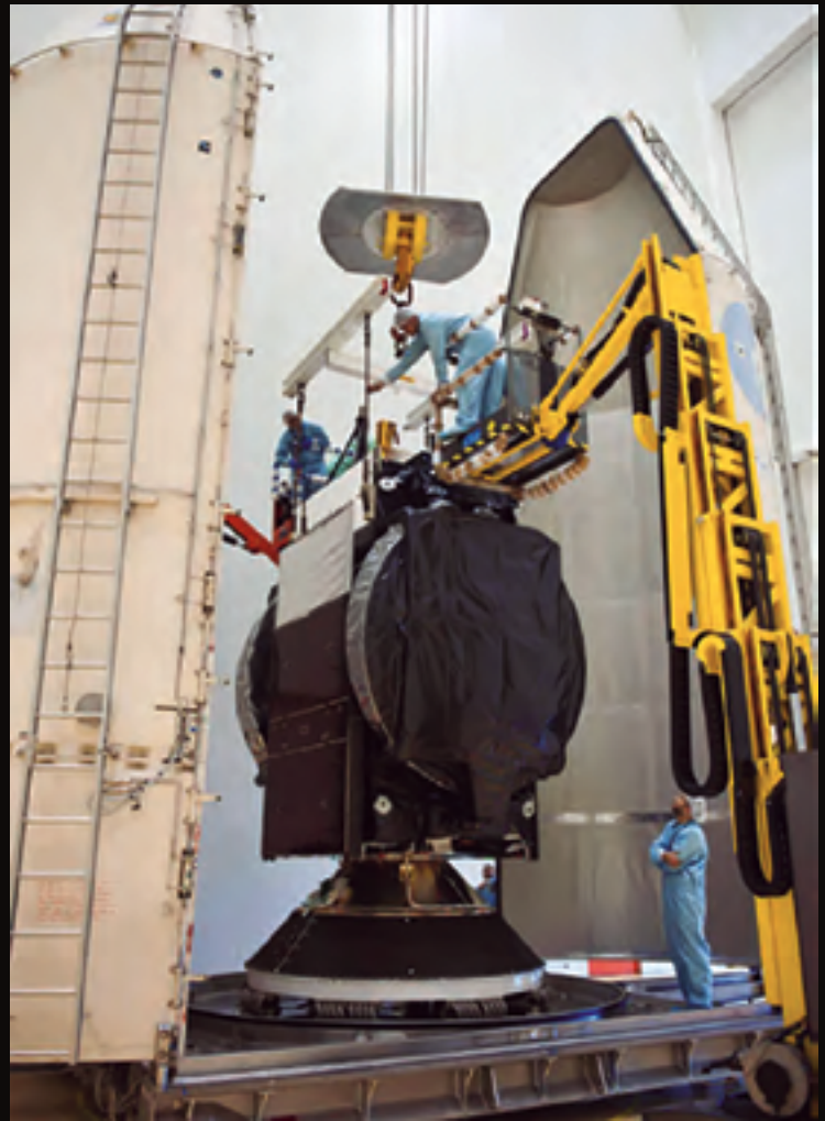
CHIRP installation within fairing.
