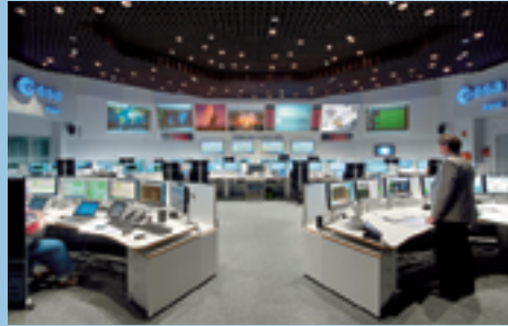
ESOC serves as the Operations Control Center for ESA missions, and hosts the Main Control Room (shown here), combined Dedicated Control Rooms for specific missions and the ESTRACK Control Center, which manages the worldwide ground tracking stations. ESOC also hosts facilities for satellite communications, navigation, networks and other special functions.
