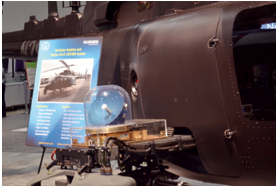
Shown at AUSA 2015, the Hughes Airborne SATCOM System featuring the new HM200 Modem installed on a NorthStar Aviation Bell 407 Multi-role Helicopter.
