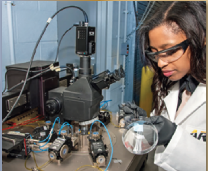
Dr. Asha Hall, a materials science engineer with the U.S. Army Research Laboratory at APG, works on the Keithly four-point probe station measuring capacitance of a light and flexible multiferroic material in a crystalline charge transfer material. Hall is a DA civilian who represents the ultimate goal of RDECOM’s STEM education and research continuum: to provide the Army with the R&D workforce it needs to win in a complex world.
