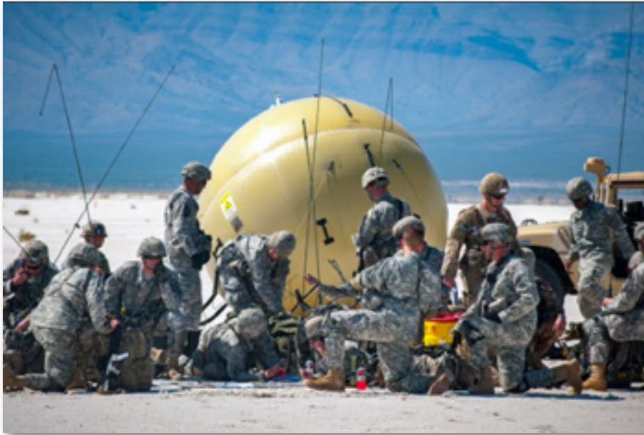
A new duo of light-weight, portable satellite terminals, called Transportable Tactical Command Communications (T2C2), will provide early entry units in air-to-land missions, as well as follow-on units at the tactical edge, with a lite (v1) and heavy (v2) variant of high-bandwidth, deployable satellite dishes, to keep Soldiers and Commanders connected to the network and well informed.
