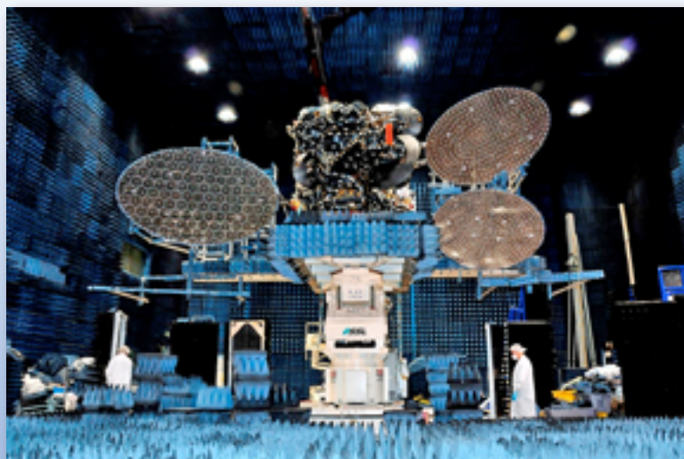
The Anik G1 satellite, built by SSL for Telesat Canada, is an FSS multi-mission C- and Ku-band GEO spacecraft designed to support a variety of applications. The satellite carries an X-band government communications payload and is the first commercial satellite to possess substantial government X-band coverage over the Pacific, ideal for naval platforms.
