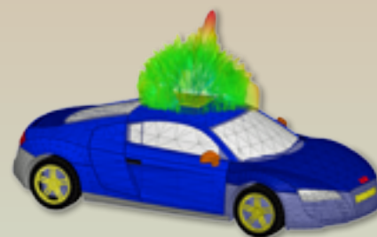
Figure 2. A flat panel array with electrical steering in both azimuth and elevation angles. Although low profile, this antenna loses gain and pattern integrity as it points off-axis
