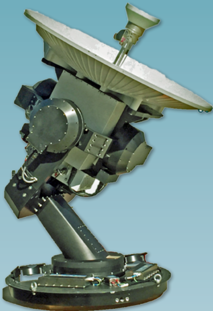
The X-/Ka-multi-band Cobra terminal houses its electronics and polarization system in an RF "can" mounted directly behind the antenna. Photo is courtesy of EM Solutions.
