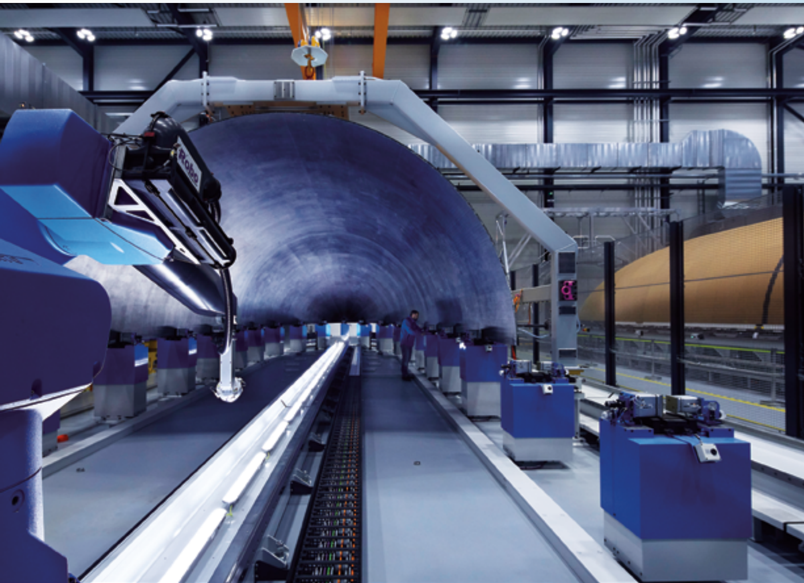
Non-destructive inspection machine. Photo is courtesy of RUAG Space.
