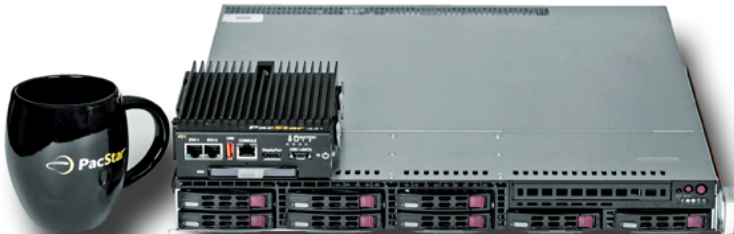
An example of the small form factor server running PKI technology as compared to a standard size server.
