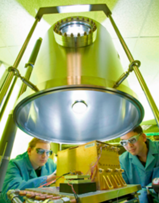
Figure 2. LGS Innovations engineers prepare a High Power Optical Amplifier for thermal vacuum testing. Image is courtesy of LGS Innovations.
