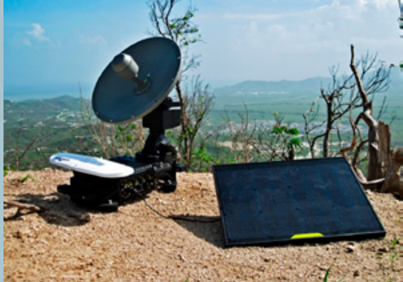
The Avwatch team used lightweight antennas, handheld radios, and solar panels to re-establish internet connectivity in Puerto Rico in the wake of Hurricane Maria Photo is courtesy of Avwatch.
