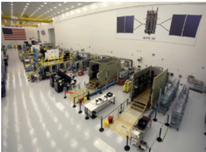
Photo of GPS III satellites in production flow at Lockheed Martin's GPS III Processing Facility near Denver. Harris navigational payloads have been delivered for the first five GPS III satellites. Photo is courtesy of Lockheed Martin.
