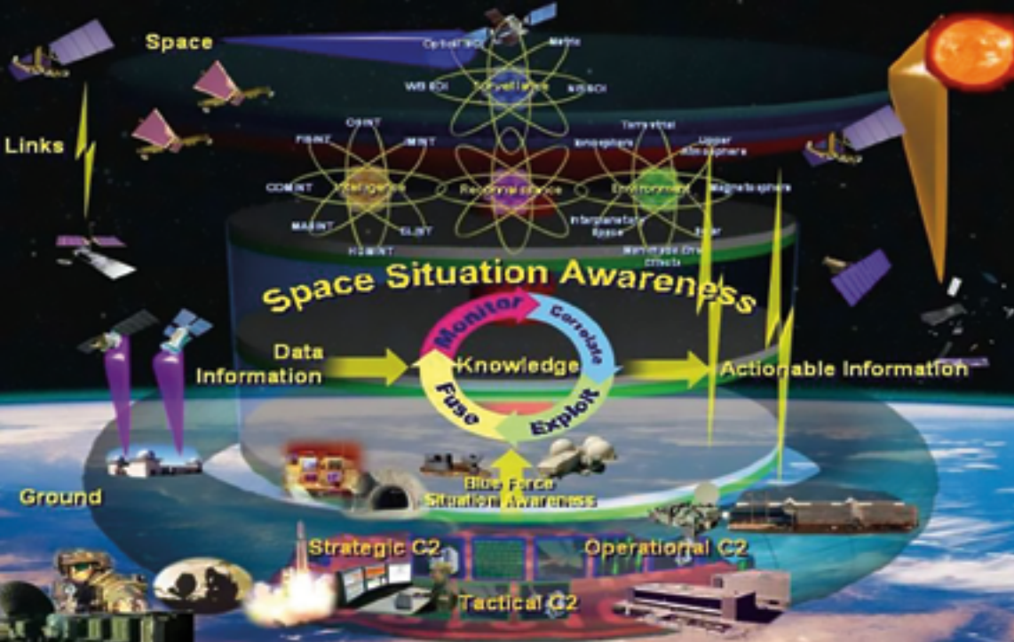
Lockheed Martin is providing the Commonwealth of Australia with an iSpace space situational awareness training and demonstration mission system. iSpace collects data from a worldwide network of government, commercial and scientific community space surveillance sensors to provide space situational awareness and space command and control. Image is courtesy of Asia-Pacific Research ( www.asia-pacificresearch.com/ )
