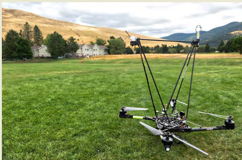
The NASA Alta X quadcopter sits in a field in Missoula, outfitted with a special structure to carry a radiosonde (sensor on the left) and an anemometer (sensor on the right) into the air. This structure was engineered at NASA’s Langley Research Center to ensure the sensors are far enough from the rotors to avoid interfering with the data collected, but without compromising the stability of the drone. Photo: NASA/Milan Loiacono
