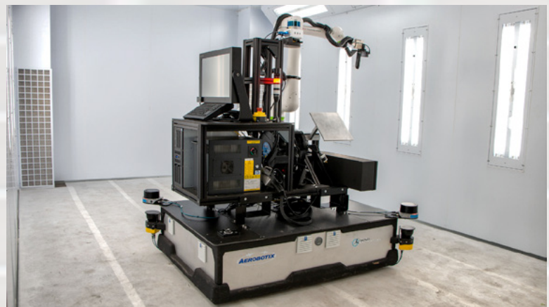
The adaptive radome diagnostic system (ARDS), the first use of a LiDAR-guided collaborative mobile robot in Air Force maintenance depots. (Photo credit: Aerobotix/CTG)
