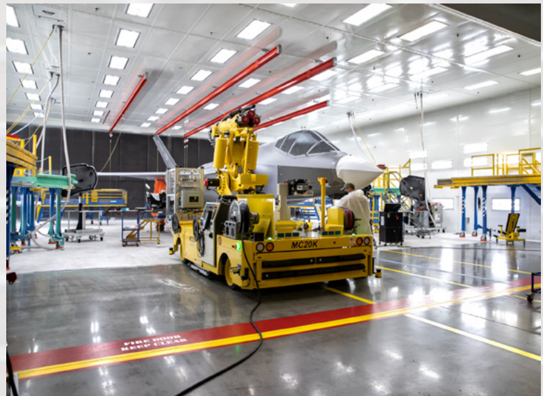
An Aerobotix robotic system applies Mold-in-Place (MIP) coatings to the side of an F-35 aircraft. (Photo credit: Lockheed Martin)
