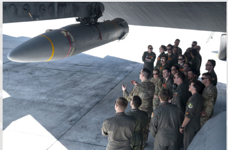
A hypersonic missile that has been sprayed with a thermal protection coating to protect the vehicle as it leaves the Earth's atmosphere. (Photo credit: U.S. Air Force)
