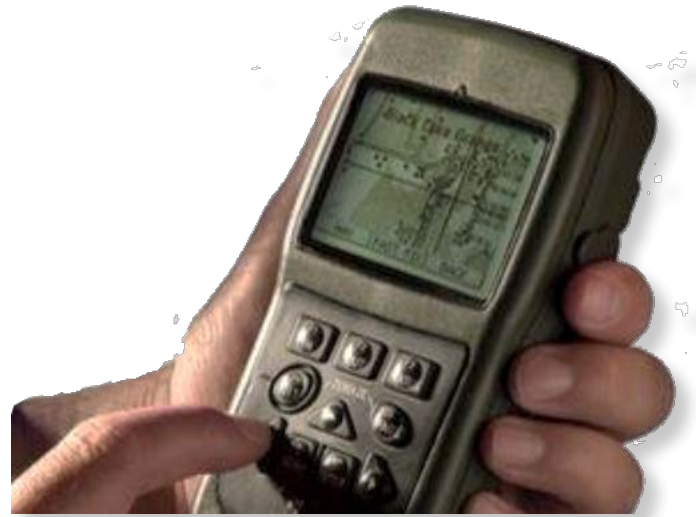
M-code enabled global positioning system receiver.
