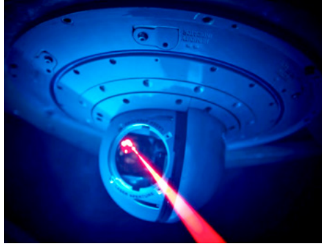
Crucial to keeping aircrews safe, LAIRCM automatically detects emerging missile threats and uses a high-intensity, laser-based countermeasure system to track and defeat missiles Photo is courtesy of Northrop Grumman.
