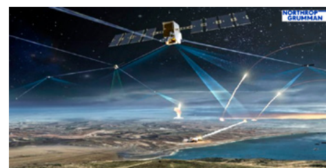
In July of last year, Northrop Grumman Corporation won a competition to build and deploy a proliferated LEO constellation of 14 satellites with infrared sensors for the Space Development Agency's (SDA) Tranche 1 Tracking Layer (T1TRK). Image is courtesy of Northrop Grumman.
