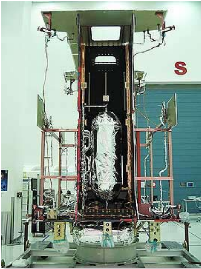
This photo is of the core propulsion module for the 2nd satellite, prior to delivery from Lockheed Martin's Mississippi Space & Technology Center to its Sunnyvale facilities in November of 2007
