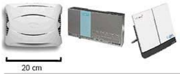
The key hardware: GSM base station, industrial PC, and satellite modem
