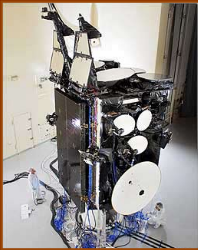
The first Advanced Extremely High Frequency (AEHF) satellite in acoustic cell testing structure at Lockheed Martin's facilities in Sunnyvale, California
