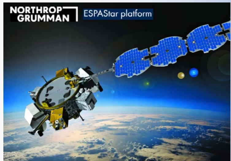
L3Harris will integrate NTS-3 using Northrop Grumman's ESPASStar bus , building on EAGLE's flight heritage.
