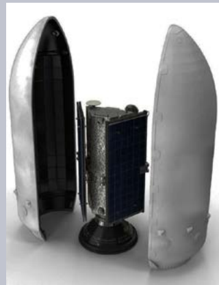
Artistic rendition of how a satellite is surrounded by the fairing, before being placed at the top of the rocket for launch.
