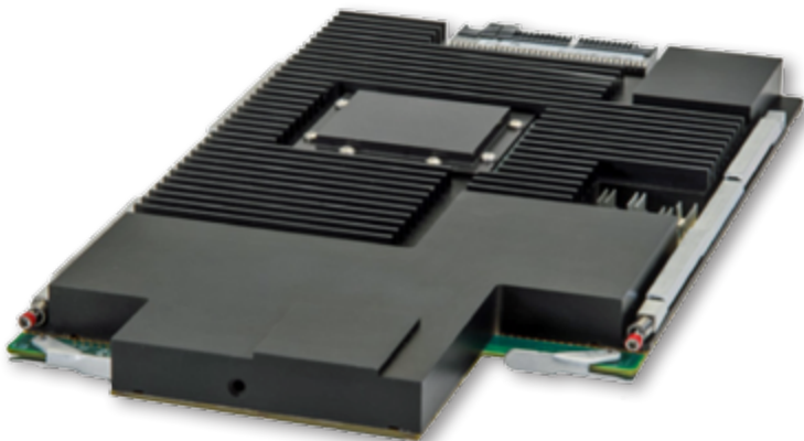
iDirect Government's 980 integrated satellite router board
