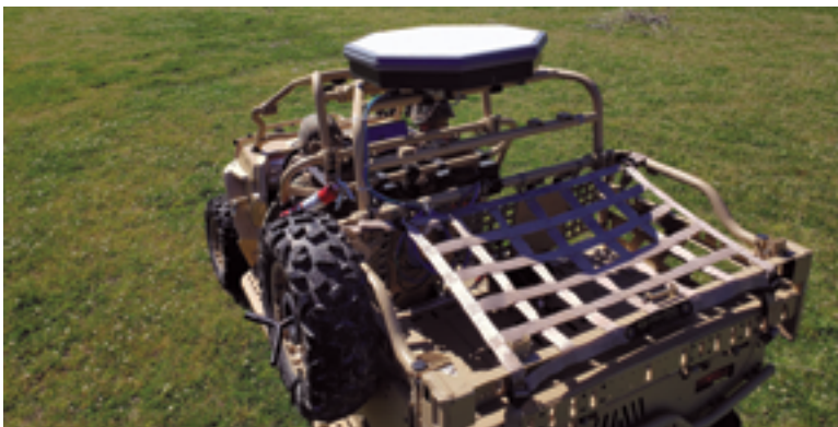
An installed CopaSAT STORM terminal.
