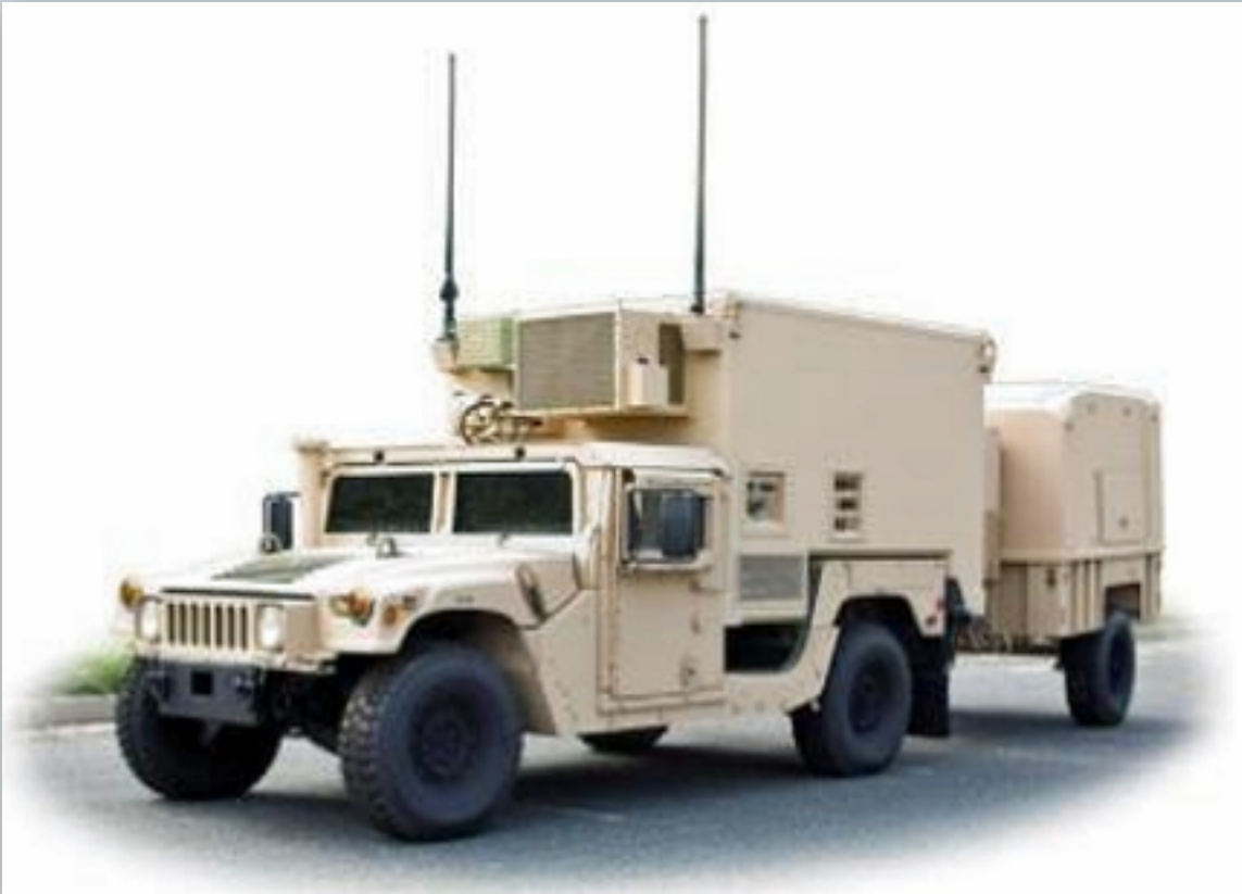
The Mobile Meteorological Facility (Replacement) Next Generation (METMF(R) NEXGEN) is a U.S. Marine Corps mobile tactical meteorological system designed in a sheltered HMMWV in support of the Marine Air Ground Task Force (MAGTF).
