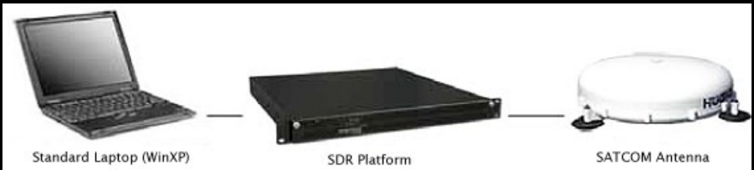
The basic components required to build a SATCOM Monitoring solution—all are COTS and software programmable.
