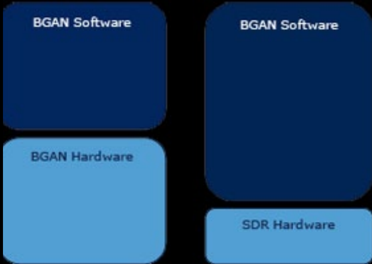
Figure 1. Using an SDR approach, the BGAN functionality is defined by software only, leaving the hardware platform generic. This is in contrast to the non-SDR approach where BGAN specific hardware is incorporated in the design.
