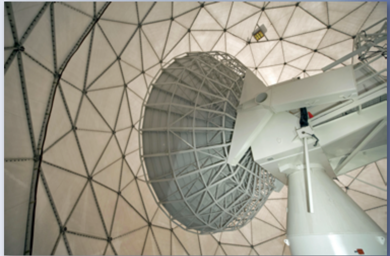
The radomes, lightly referred to as "golf balls," on Buckley Air Force Base, Colorado, house and protect satellite dishes and other crucial space operations equipment. The purpose of the giant spheres is to protect the equipment from the weather. Photo is courtesy of US Air Force / Airman 1st Class Emily E. Amyotte.
