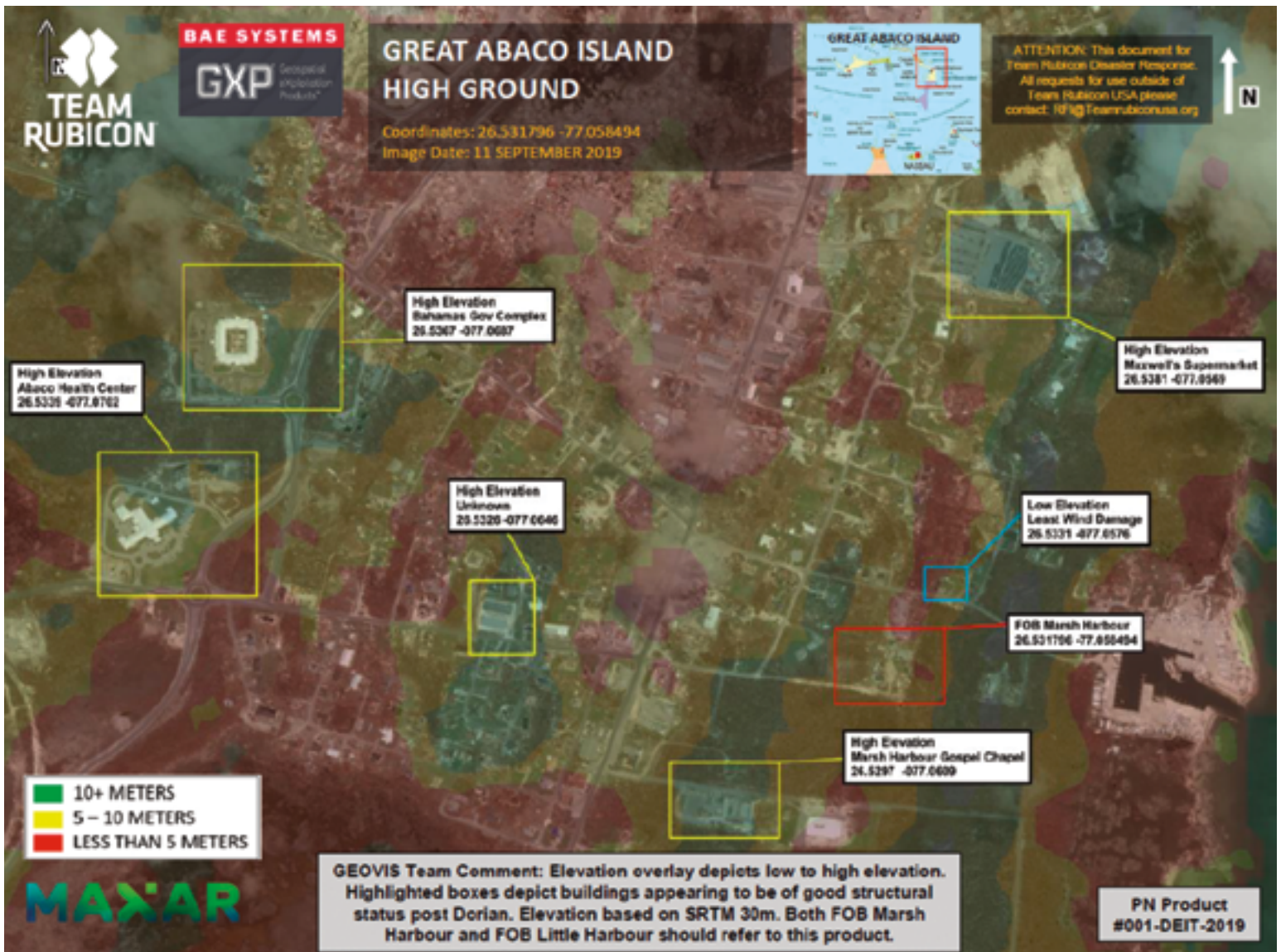
This visual shows part of an imagery product produced by a Team Rubicon GeoVis analyst that identifies buildings of good structural status and high elevation on Abaco Island, The Bahamas. This was used for contingency planning and identified hardened locations for our deployed teams to evacuate to should a storm threaten the island.
