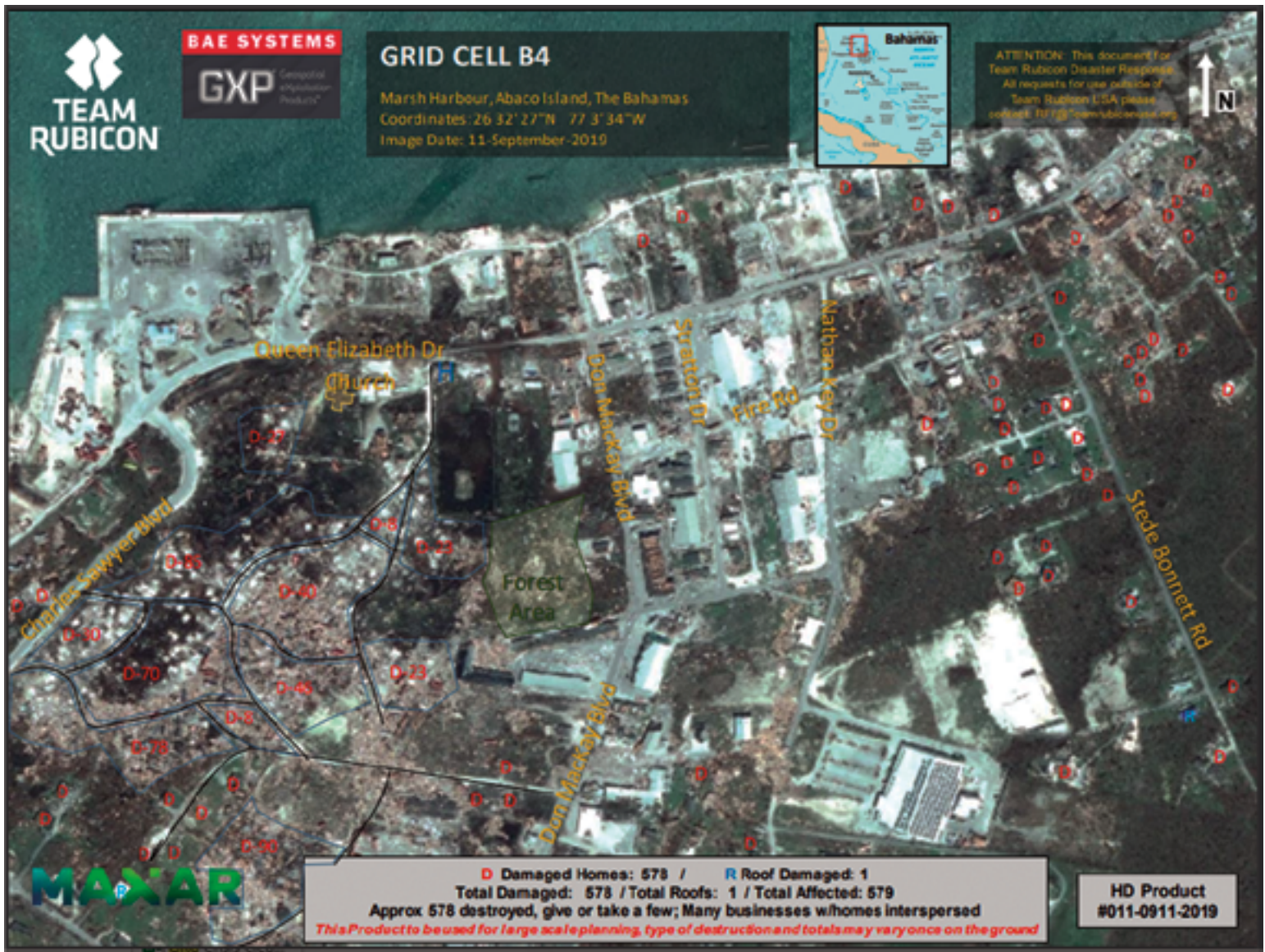
This image shows part of an imagery product produced by a Team Rubicon GeoVis analyst over the town of Marsh Harbour on Abaco Island. The analyst used a Maxar WorldView-3 image collected after the hurricane hit the town and used GXP WebView to identify and annotate damaged homes and roofs.
