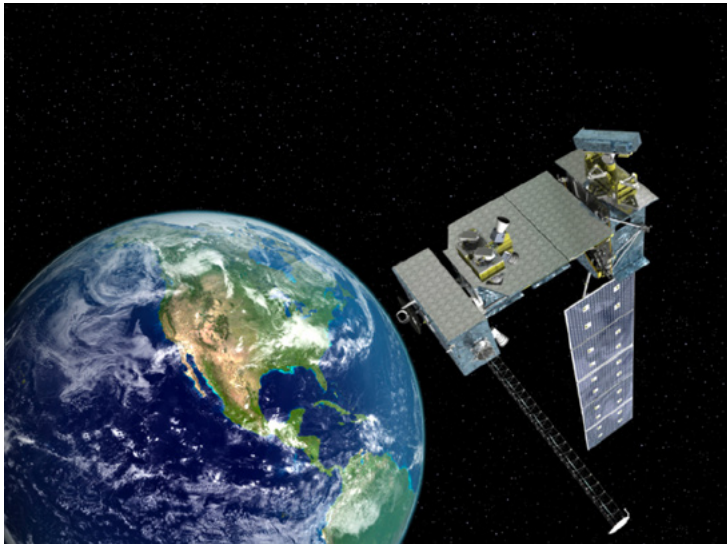
STPSat-6's nine payloads include the National Nuclear Security Administration (NNSA)'s Space and Atmospheric Burst Reporting System (SABRS), NASA's Laser Communications Relay Demonstration (LCRD) and seven Space Experiments Review Board (SERB) payloads that demonstrate cutting edge space technologies. Artistic rendition is courtesy of Northrop Grumman.
