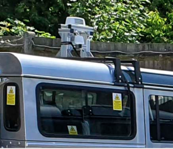
Photo of a roof mounted, Blu Wireless node.
