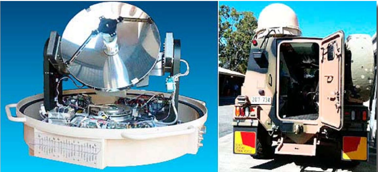
Figure 1: Views under the radome, and mounting to the Bushmaster PMV
