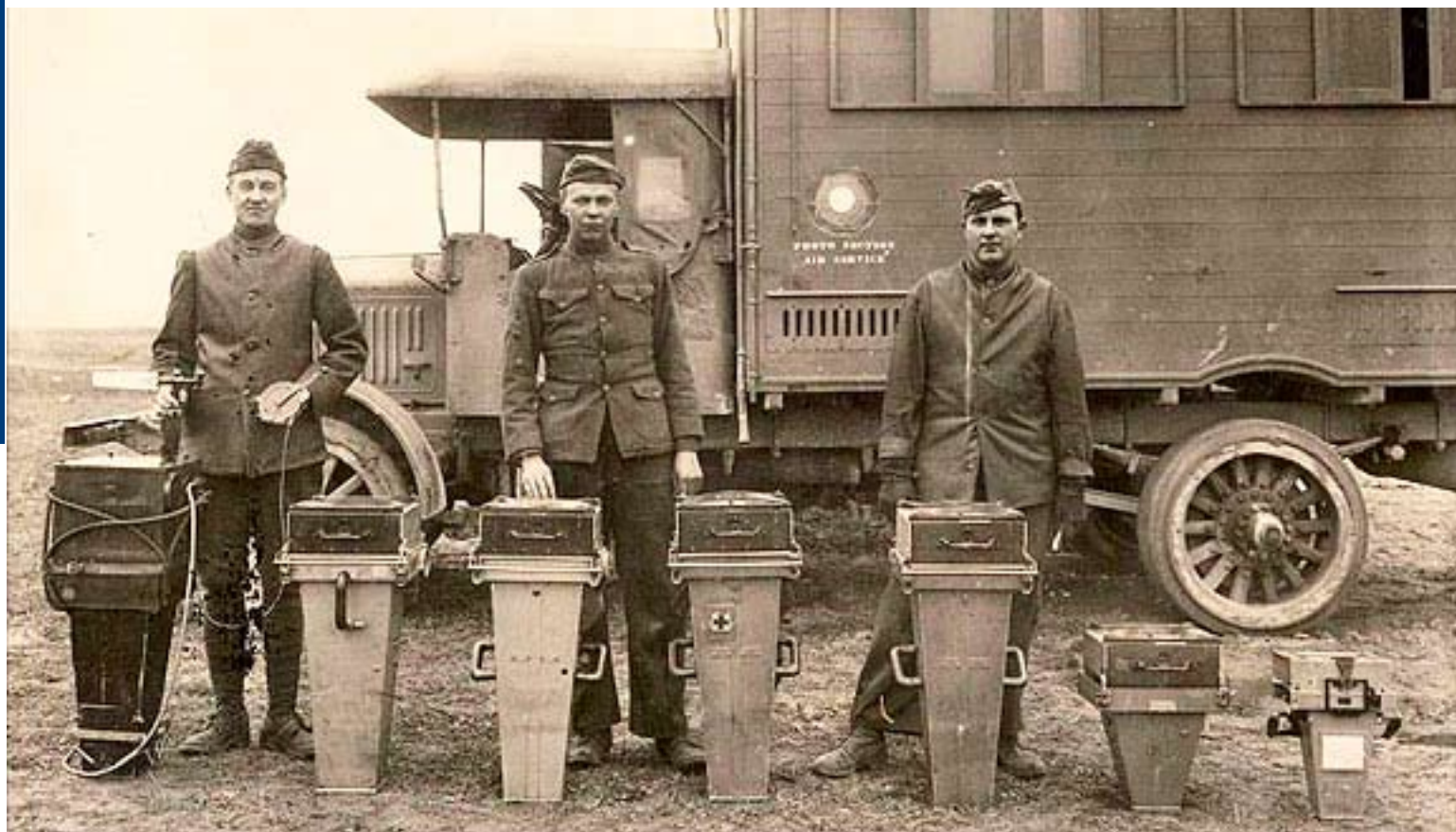
1914 camera photo reconnaissance cameras...the pilot held the huge camera over the side of the plane and acquired photos from approximately 12,000 feet in the air. Photo courtesy of The History Blog.
