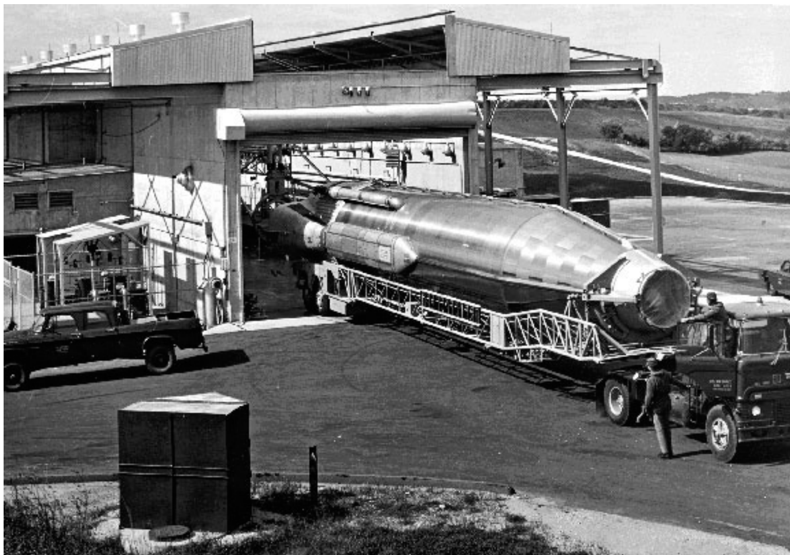
An Atlas D missile being trailored for its move from its above ground launcher.
