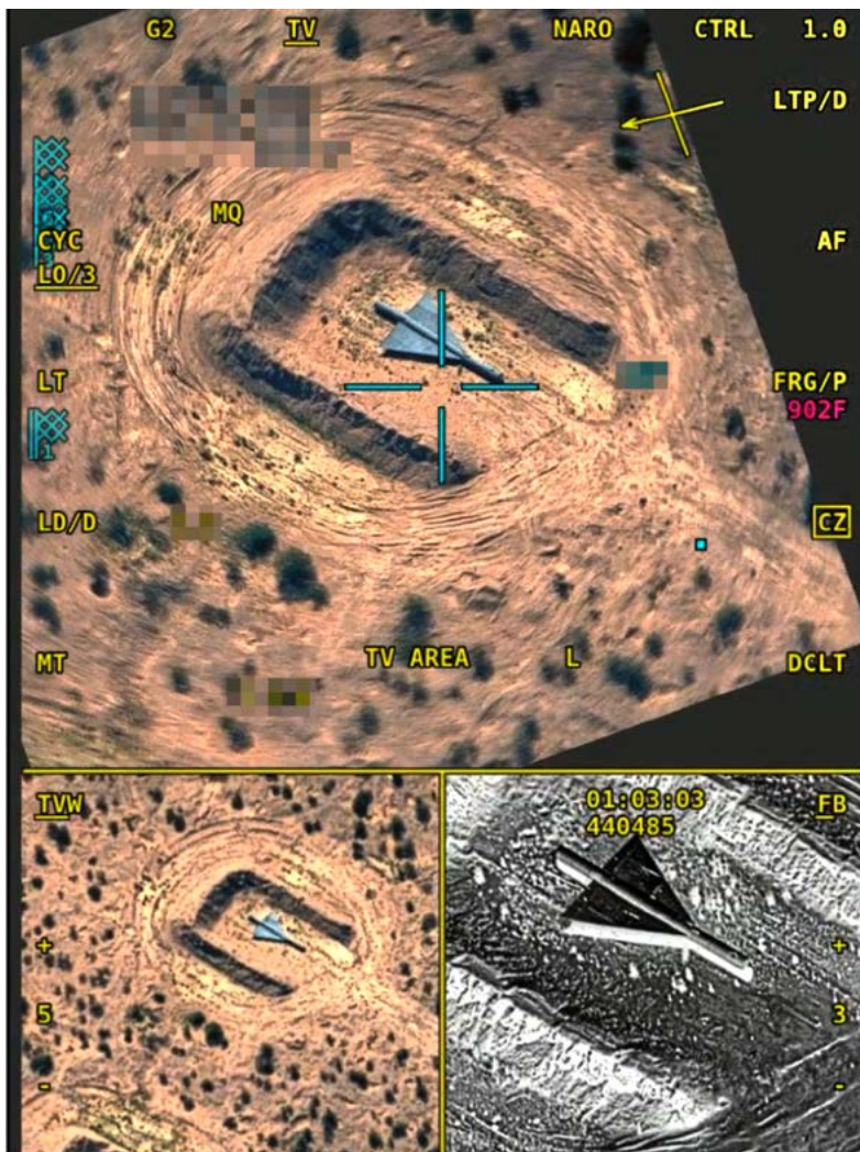
LITENING is an electro-optical infrared sensor system for targeting and surveillance that enables aircrews to detect, acquire, identify and track targets at long ranges. LITENING enables a wide range of missions, including precision targeting, close air support, intelligence, surveillance and reconnaissance, and humanitarian assistance.
