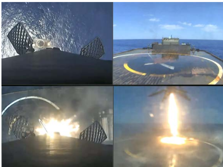
Screen captures are from the SpaceX live stream of the launch and shows the droneship before and after the Falcon 9 first stage completes a successful landing.
