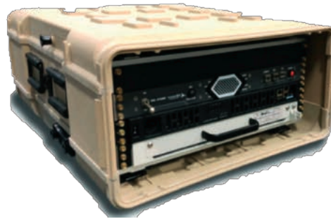
From left to right: Shoulder panel mount - RORO transit case with iDirectGov 9800 AR - Hatch mount without radome
