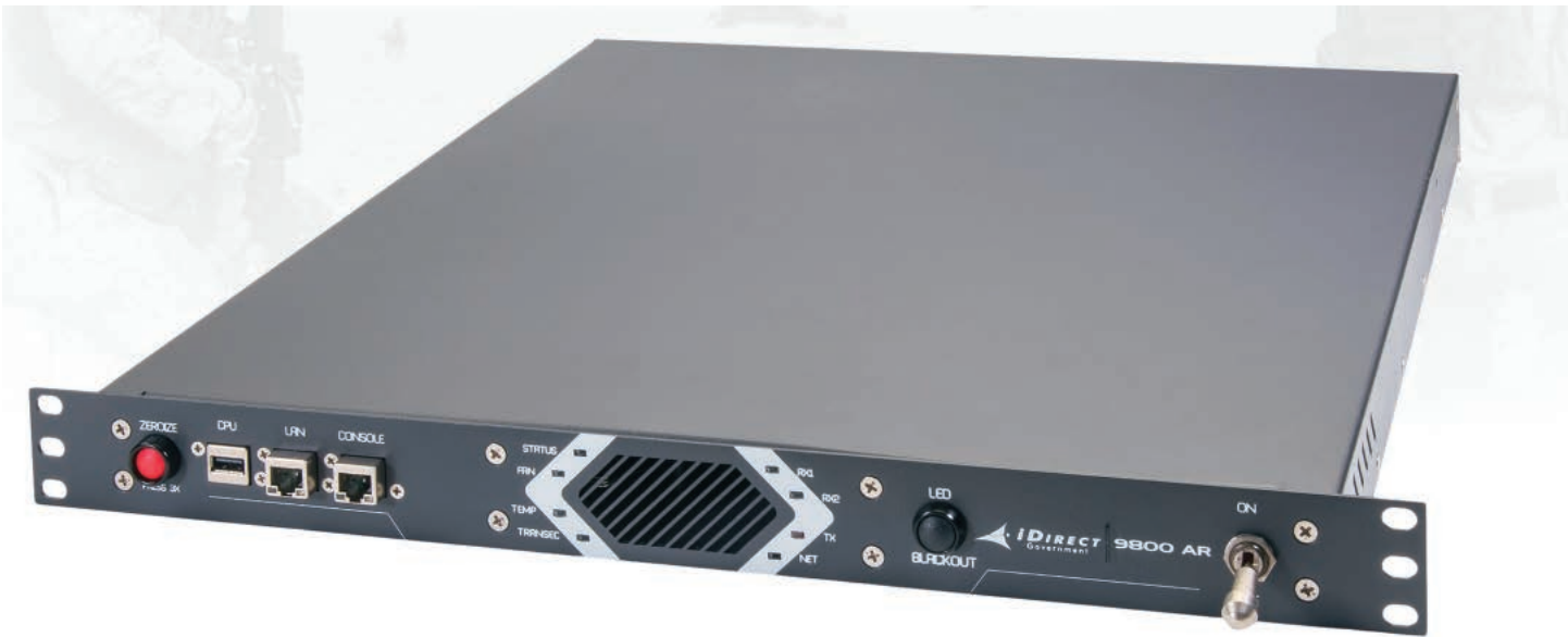
iDirectGov's 9800 AR Airborne Satellite Router.
