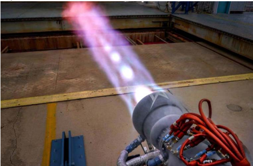
The Masten 25k lbf thrust Broadsword rocket engine. Photo/Matthew Kuhns.
