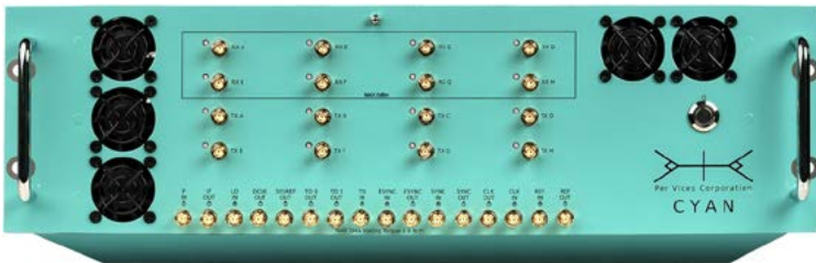
Figure 3: Per Vices's Cyan is an SDR with a storage solution.
