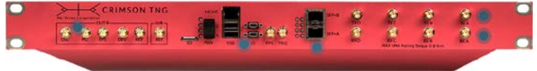
Figure 4. Crimson TNG offers a 4 receive and 4 transmit radio chain architecture that supports independent control on each of the radio chain or the ability to share a common LO for better phase coherency and stability performance. Each radio chain has an impressive 325 MHz of bandwidth with 16 bit converters and a tuning range from near DC to 6 GHz. The digital interface for controlling the system is a standard 1G Ethernet port and the data transfer is done over dual 10GBASE-R interfaces, providing users with up to 20 Gbps of data transfer.
