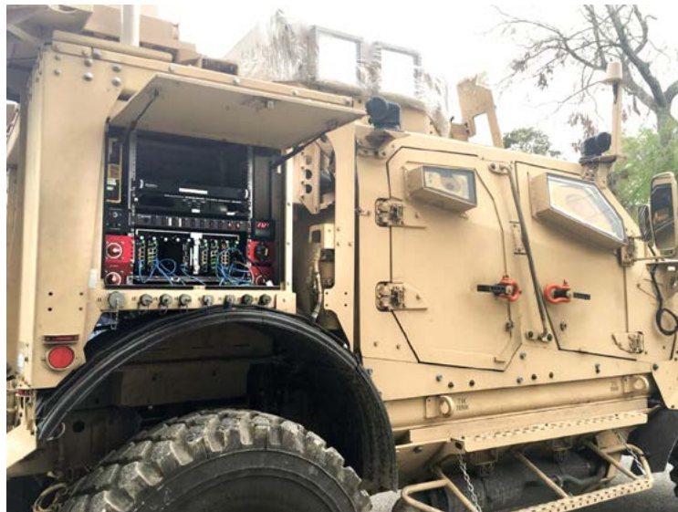
Figure 6. Rugged PacStar communications equipment mounted on a U.S. Marine Corps JLTV
