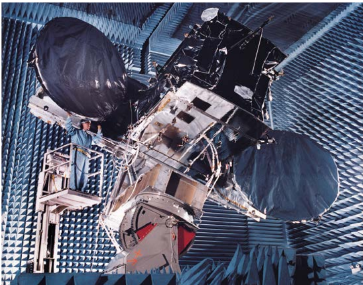
Photo of Lockheed Martin's a2100 satellite bus during manufacturing.
