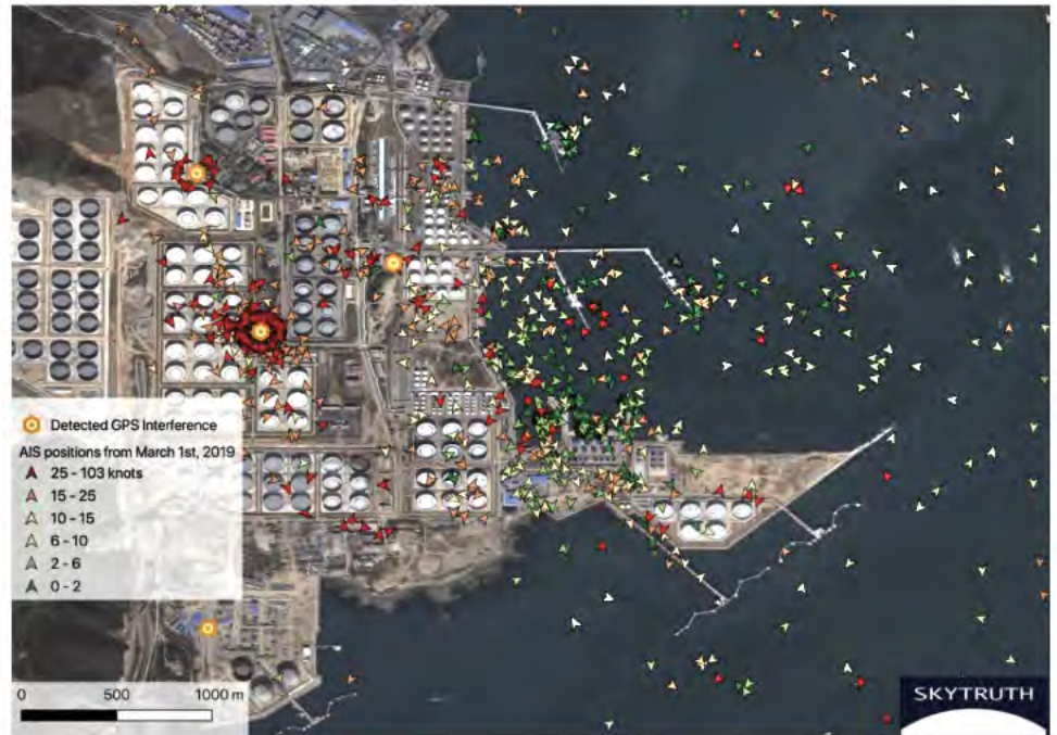
Figure 4 (above): GPS Crop Circles Near Dalian China. Research organization Skytruth found that two GPS interference locations around an oil terminal were active and had a dramatic effect on scrambling vessel positions in the area on September 5, 2019. Some vessels were even shown to be far inland. “On the water many positions are appearing with very high speeds (over 25 knots, red) and it’s not possible to distinguish true and false locations. However, some slow speed GPS positions (green) are appearing at dock where they would be expected, so some AIS broadcasts appear to be unaffected.”
