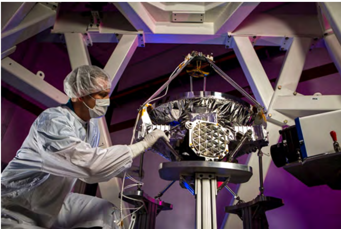
A Raytheon Intelligence & Space engineer works on the Infrared Imaging Space Experiment, or IRISX. Electronics play a critical role in a sensor's ability to gather and process data.
