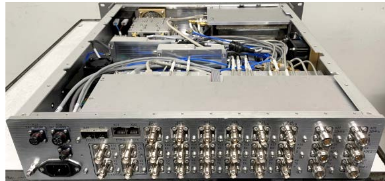
Figure 4: The Cobra Antenna Diversity System viewed from the rear, showing the switch matrices internally and connectors for multiple modem connections on the rear panel.
