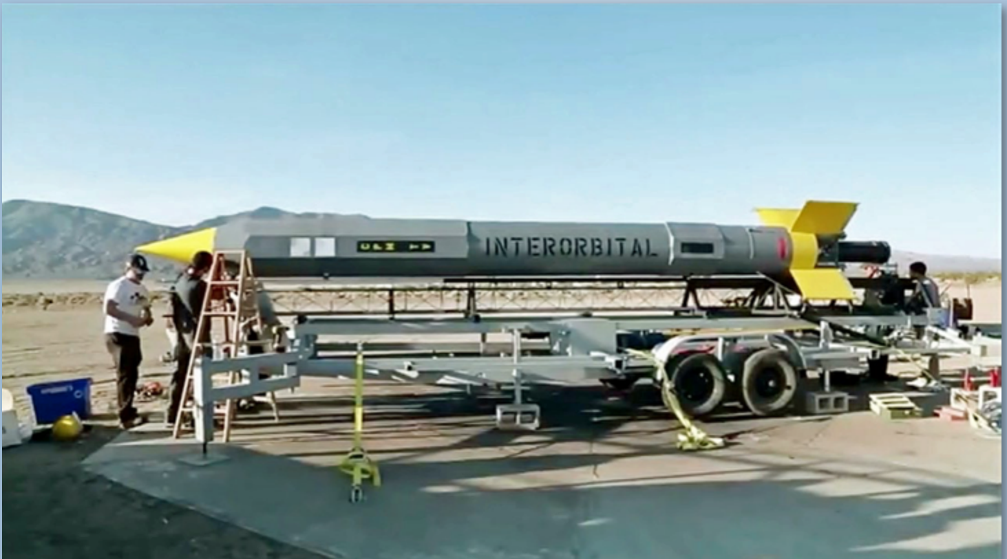
A single Common Propulsion Module (CPM) sounding rocket on its mobile launcher. Bundling three of the CPMs produces the Neptune (N3) orbital rocket.
