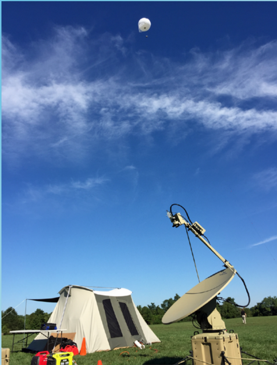
The new TPS—or Tactical Persistent Surveillance—solution takes an inflatable aerostat platform, many of which are in use across the globe for reconnaissance, and adds connectivity via the SES satellite constellation. Photo is courtesy of SES.
