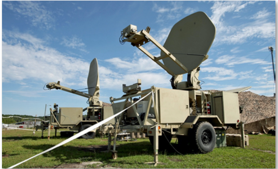
Two Very Small Aperture Terminals (VSAT) Large, are positioned during a field exercise conducted by Alpha Company, Marine Wing Communications Squadron 28. USMC photo by Cpl. Jason Jimenez.
