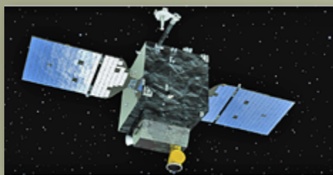
Orbital ATK's GEOSTAR-1 is the platform of the SPTSat-6 primary space vehicle for the STP-3 mission.
