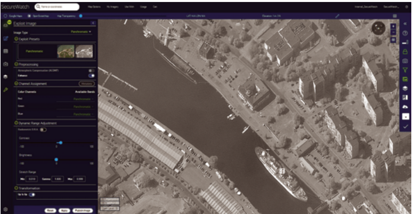
Figure 7. This recent WorldView-1 image of Kaliningrad was not used for mosaic production because it is panchromatic (black and white) and was collected at a high off-nadir angle. This image is still very valuable for an analyst studying facilities this area and is available in SecureWatch both online and with Image Exploitation Mode.
