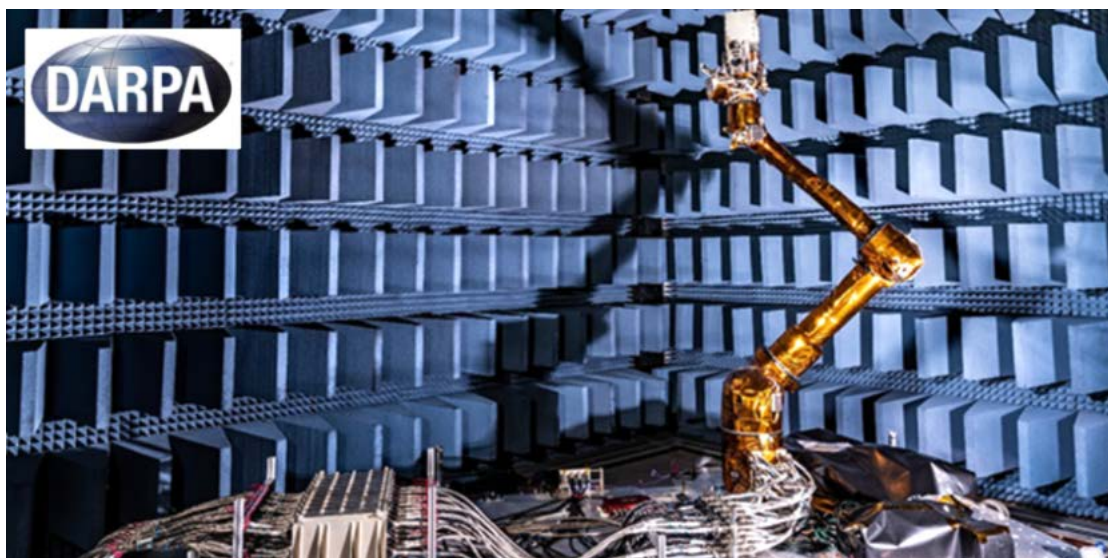
Flight manipulator arm, part of the RSGS robotic payload, in electromagnetic test. Image courtesy NRL.
