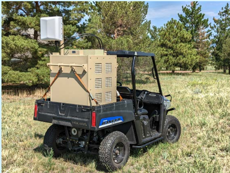
SEMPRE offers distributed micro edge datacenters that ensure access to data with highly secure connectivity and high-performance compute in a fixed location or on-the-move—all in a tamper-resistant, EMP-hardened enclosure. Pictured: SEMPRES T "transportable" micro edge datacenter.
