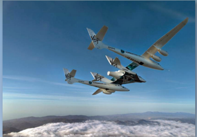
Photo of Virgin Galactic's ‘captive carry’ flight test, during which VSS Unity remained mated to the firm's WhiteKnightTwo mothership (VMS Eve) for the entire flight, from takeoff to landing. Photo is courtesy of Virgin Galactic.
