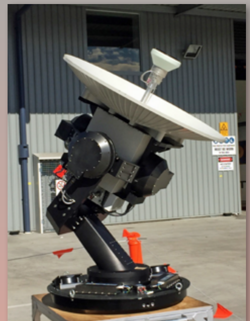
Figure 5. Under the cover — the Cobra multiband X-/Ka- terminal in test at the EM Solutions factory
