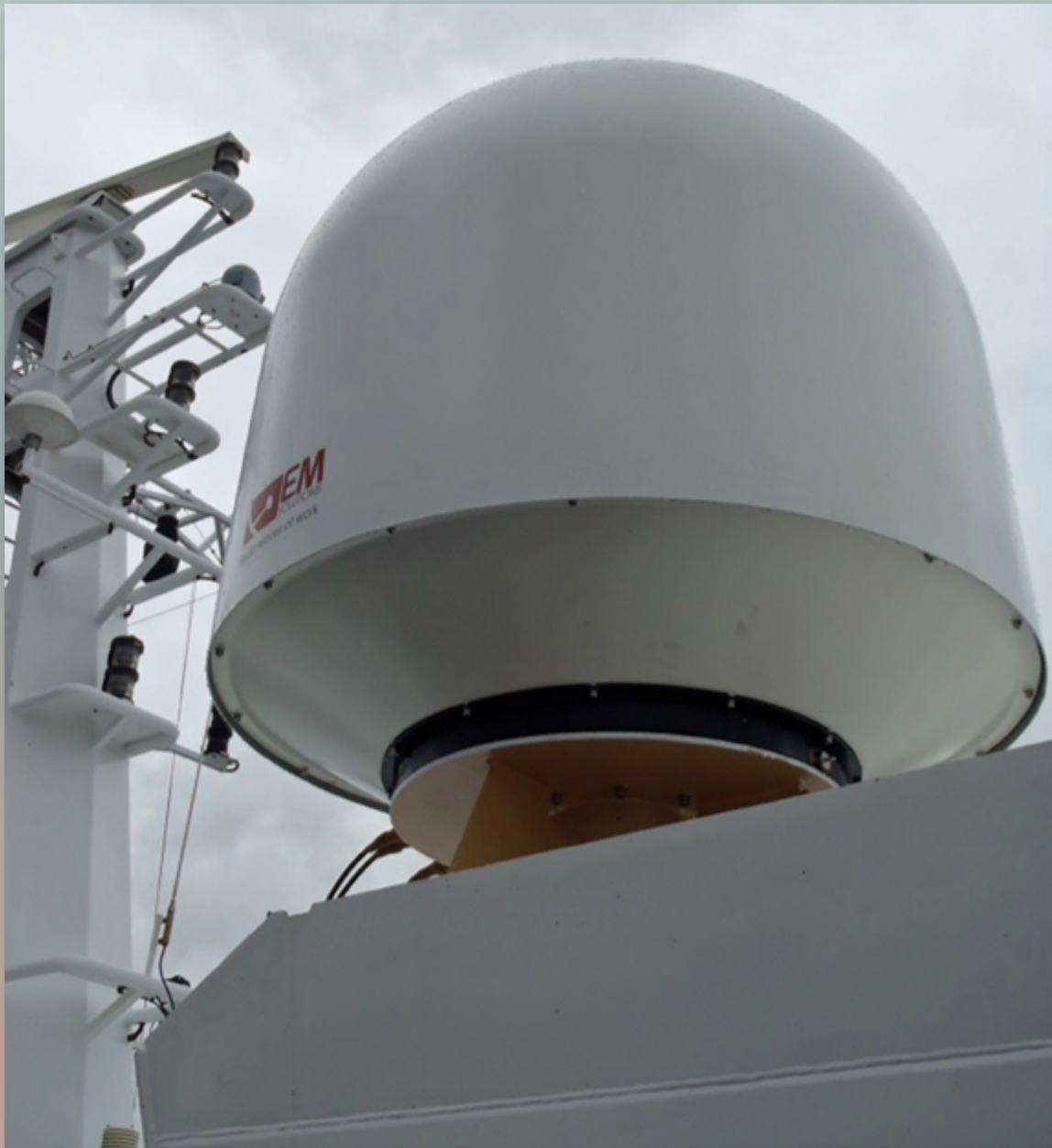
Figure 3. The first of the Ka-multiband terminals on board an Australian Border Force vessel.
