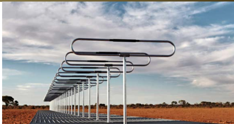
The Silentium Defence MAVERICK S-series passive radar system for surveillance of space.
