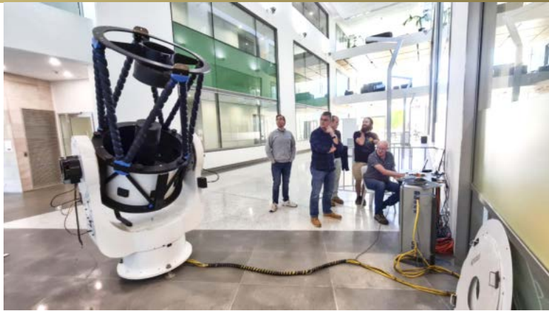
The 0.7 meter optical telescope donated by Colin Eldridge that will be used for the ground station.
