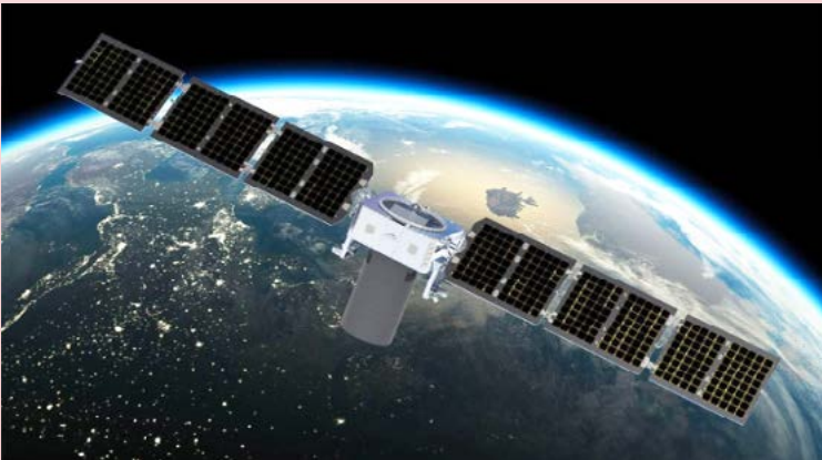
Small satellite constellations can be built from satellites such as Blue Canyon Technologies’ High Performance Commercial X-SAT Saturn ESPA-grande spacecraft, shown here. Constellations can improve the speed of sensing and reduce latency.
