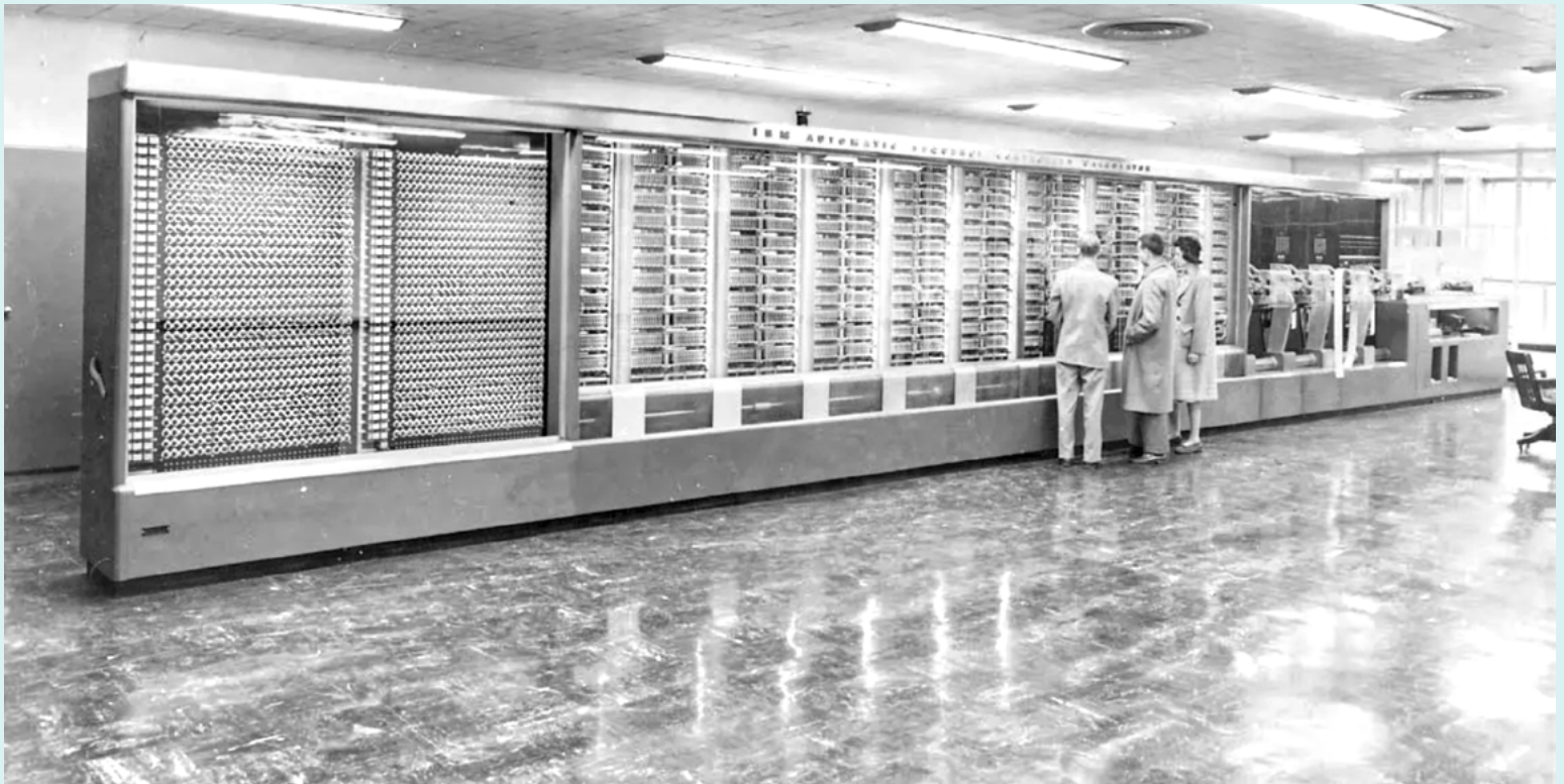
Designed by Howard Aiken, this electromechanical computer, more than 15 meters (50 feet) long and containing some 750,000 components. This computer was used to make ballistics calculations during World War II. Photo: IBM Archives.
