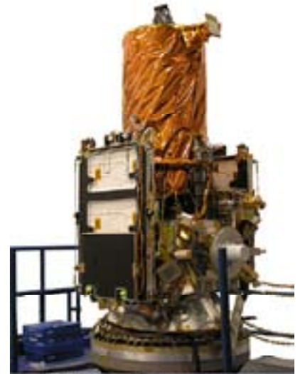
TacSat-2 spacecraft during vibration testing at Kirtland Air Force Base, N.M.
