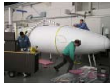
Closeout activities on the upper launch stack
