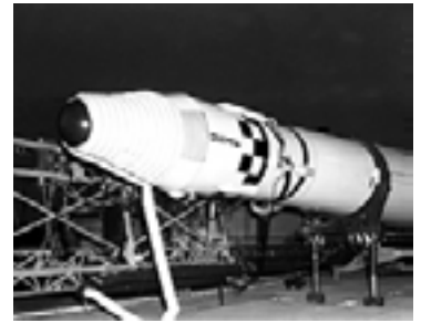
The Agena spacecraft for Discoverer 13, mated to its Thor launch vehicle, at Vandenberg AFB
