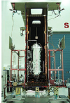
The second AEHF satellite's core propulsion module Photo: Lockheed Martin Space System
