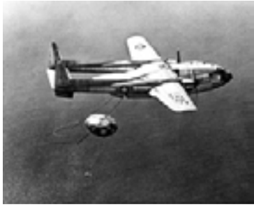
A recovery crew of the 6593rd Test Squadron (Special) performs a midair capsule recovery in a JC-119 aircraft
