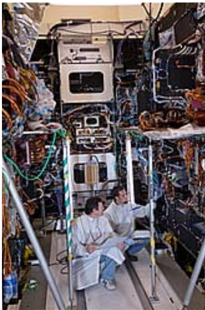
In February of 2007 employees at Northrop Grumman Space Technology in Redondo Beach, California, conduct final test and inspection of the payload module for the first Advanced Extremely High Frequency (AEHF) military communications satellite
