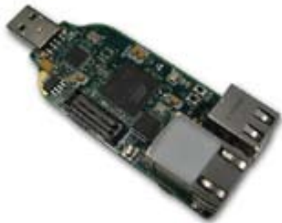
PEP-on-Stick™ by Global Protocols illustrates the trend toward lightweight, low-power accelerators
