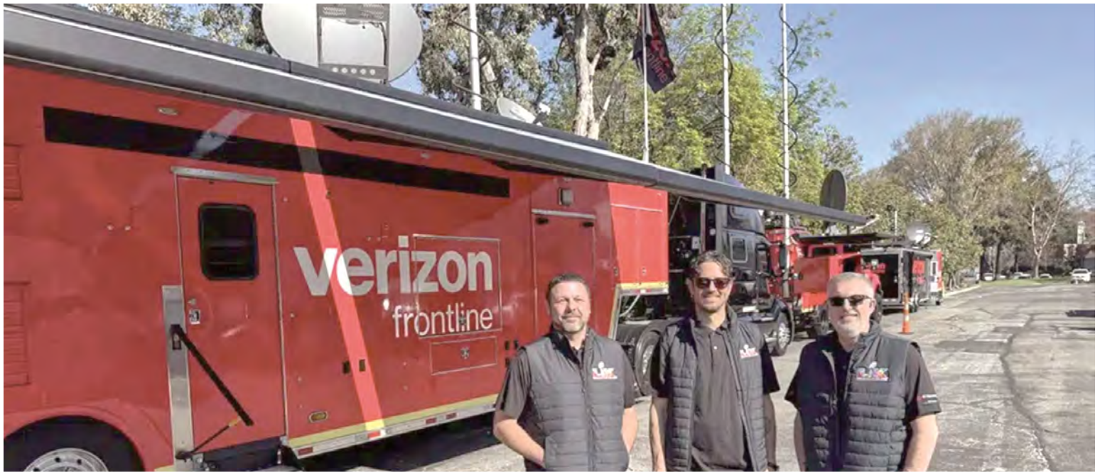
Satellite Picocell on Trailer (SPOT): A deployable solution that supported up to 400 users with satellite backhaul and Wi-Fi access, ensuring connectivity in remote or high-demand areas. Photo courtesy of iDirect and Verizon Frontline.
