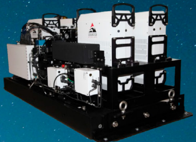
4kW Redundant SSPA System for Artemis II
